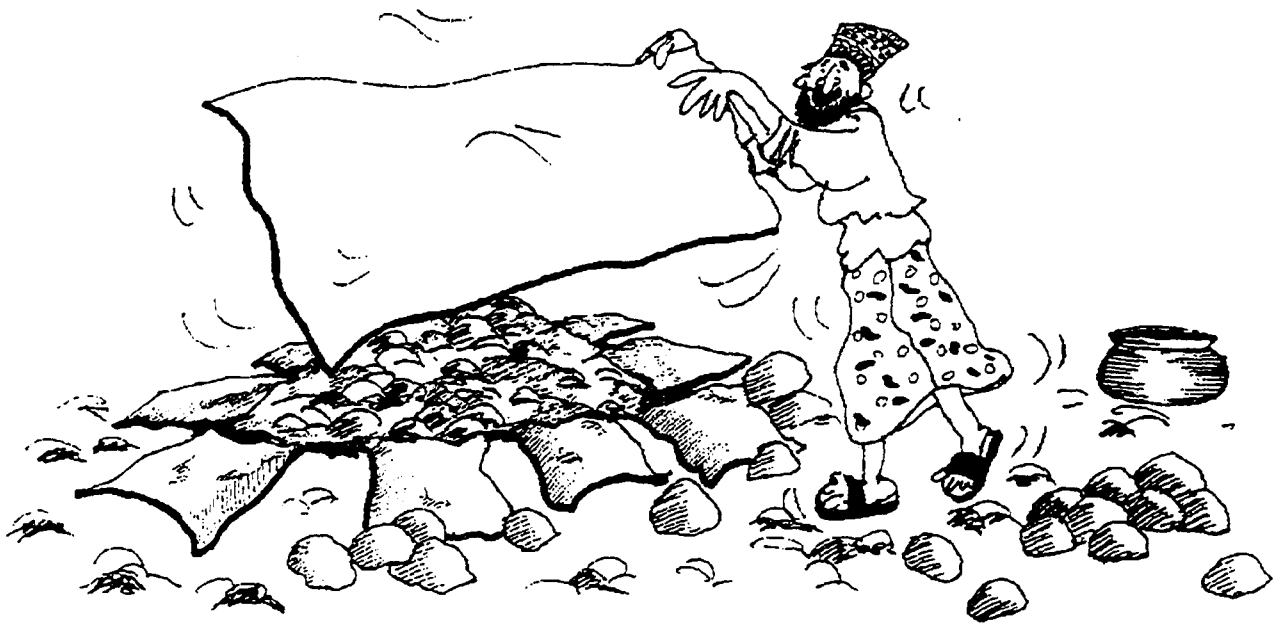
Storing the clay in a pit and covered with plastic sheets
