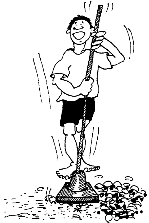
Crushing clay with a heavy piece of metal attached to a stick
