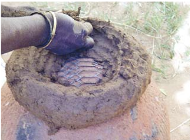
Pic 63. The mixture is formed into a circle and pressed on to the grill.
