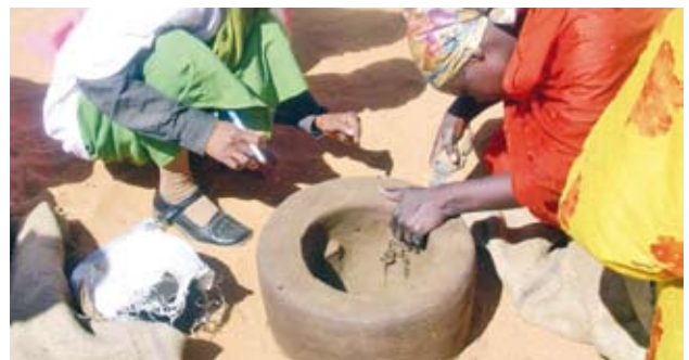
Pic 60. This exhaust hole increases the stove efficiency by increasing the air flow. It also allows wood to be added without the need to move the saucepan. The stove should be left to dry naturally, it does not require burning.
