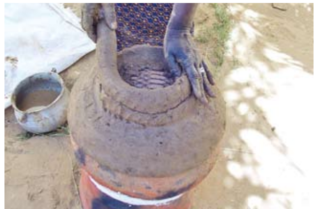
Pic 65. Layers of clay are used to build up the stove walls.
