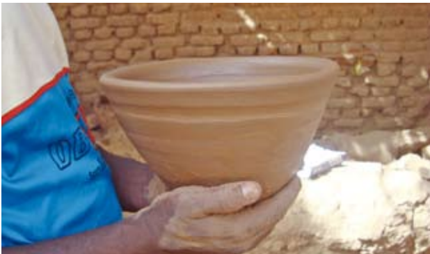
Pic 27. The vessel is removed from the wheel bat by hand or by using a knife. It is then left in the sun to dry a little, normally between 1/2 hour and an hour depending on the weather.
