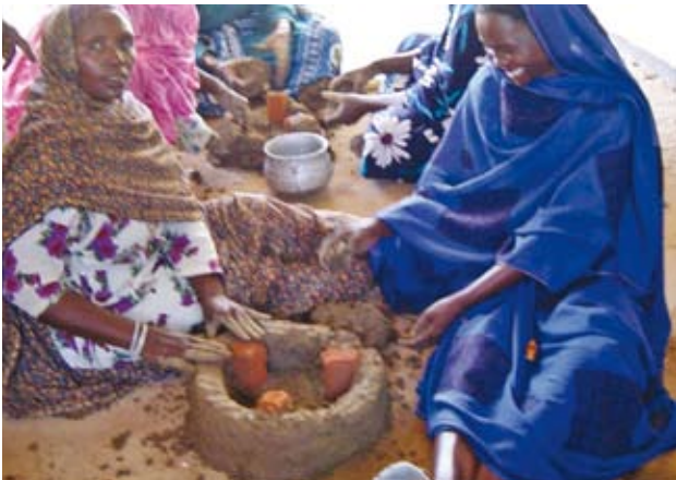
Pic 57. The walls are then built up outside the bricks although a small part of the bricks are embedded in the wall. The walls are roughly 4cm thick. The wall is built up until it is flush with the top of the bricks.
