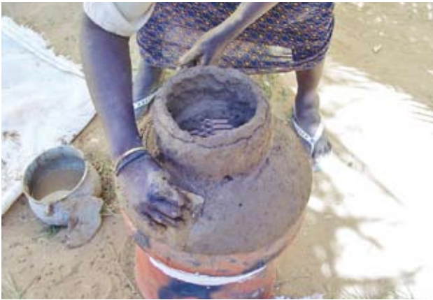
Pic 66. The chamber walls are finished and the surface is smoothed.
