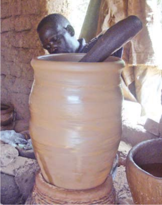
Pic 36. Further clay is added to increase the size of the vessel and the rim is formed.
