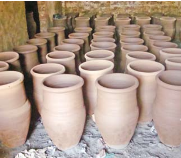
Pic 37. The completed zeer pots are stored indoors for one day to dry slowly to prevent shrinkage after that they are left in the sun for a further day.
