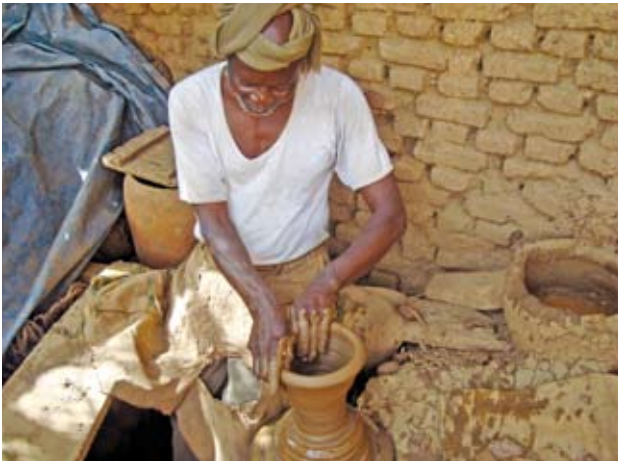
Pic 25. The hole is then widened. The sides thus defined are pulled up and made thinner by pressure between the hands.
