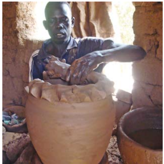
Pic 35. Further clay is added to increase the size of the vessel (The same process as shown in pictures 28 - 31).
