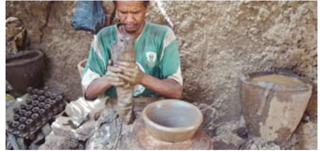
Pic 28. The vessel is placed in the former (this piece of equipment is secured to the wheel bat and holds the vessel) and a new piece of material is prepared.
