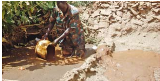
Pic 21. The filtered clay hole is then drained of water which goes back into the mixing hole leaving behind good quality clay ready for use.
