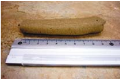
Pic 8. In this example the clay had shrunk to 93 mm a shrinkage rate of 7% which is acceptable.
