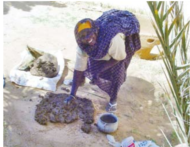
Pic 72. The base of the stove is formed by adding clumps of clay.
