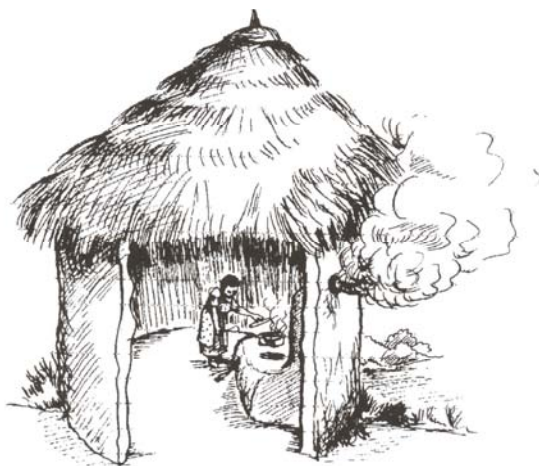
Figure 3.17 The chimney may be directed at the highest point of the wall
