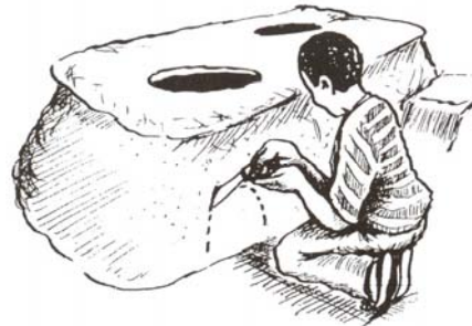
Figure 5.31 Cutting out the door
