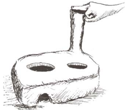
Figure 3.15 Ensuring the chimney diameter is correct
