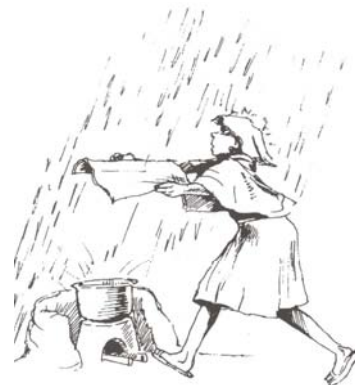
Figure 2.7 Mud stoves require shelter from the rain
