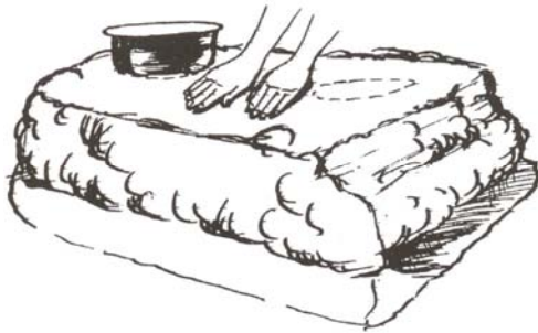
Figure 5.28 Marking the Pot-holes position
