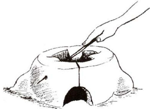
Figure 5.68 Making a smoke vent
