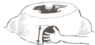
Figure 5.66 The height of the stove door
