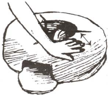
Figure 3.5 Measuring the wall thickness
