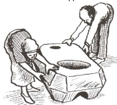
Figure 5.43 Fixing the top of the stove
