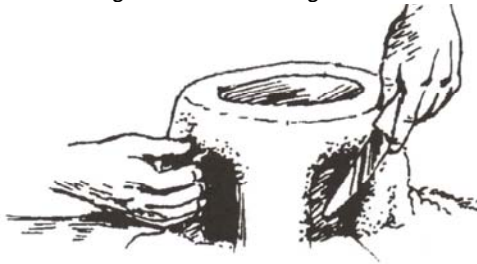
Figure 5.15 Cutting out the doors
