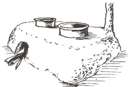
Figure 3.1 Thick walls improve performance of stoves
