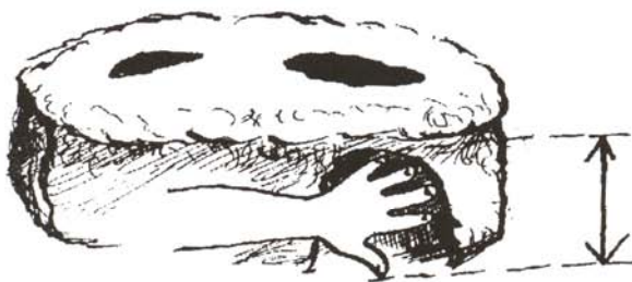
Figure 5.70 Height of the stove door
