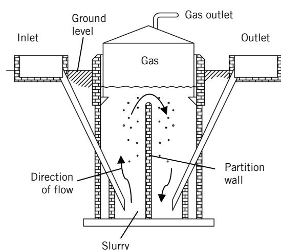
Figure 2: Floating cover digester
