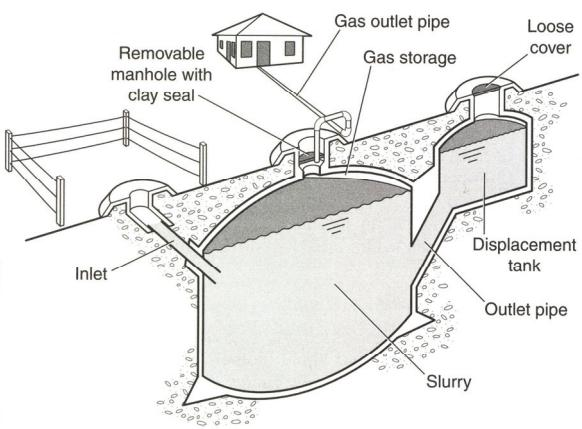
Figure 1: Fixed dome digester
