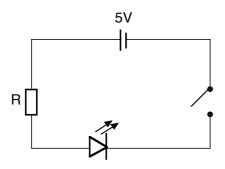
What value of resistor will see the LED radiate the brightest?
