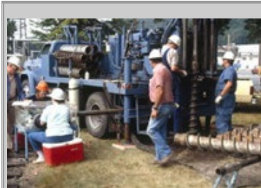
U.S. Environmental Protection Agency scientists collecting aseptic core samples using a specialized auger rig and a nitrogen-filled field glove box (circa 1989).
