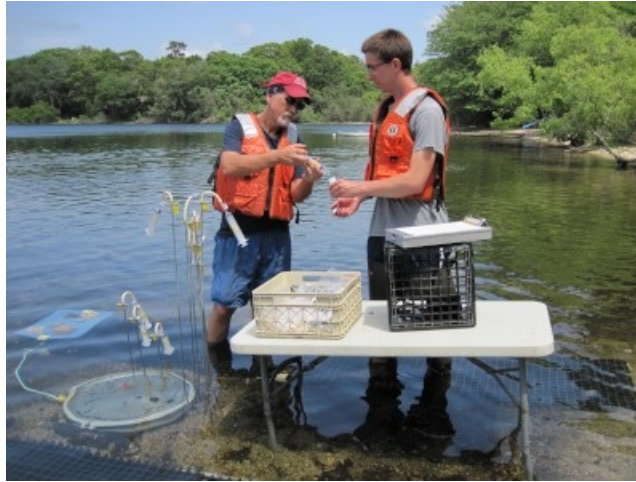
USGS scientists collecting water-quality samples from shallow groundwater under Ashumet Pond, Cape Cod, Massachusetts. USGS scientists determined that the colmation layer (top 25 centimeters of lake sediments) was highly effective in removing cyanobacteria, viruses, and dissolved organic carbon during water passage through the lake bottom to aquifer sediments. Photo Credit: Denis R. LeBlanc, USGS
