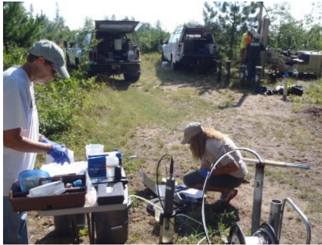
U.S. Geological Survey (USGS) scientists collecting a groundwater sample from a well at the USGS Bemidji Crude-Oil Spill Research Site, Minnesota. The scientists monitored in real time the dissolved oxygen, pH, specific conductance, and temperature of the water as the well is pumped so they can know when to collect a representative sample. Photo Credit: Jared Trost, USGS
