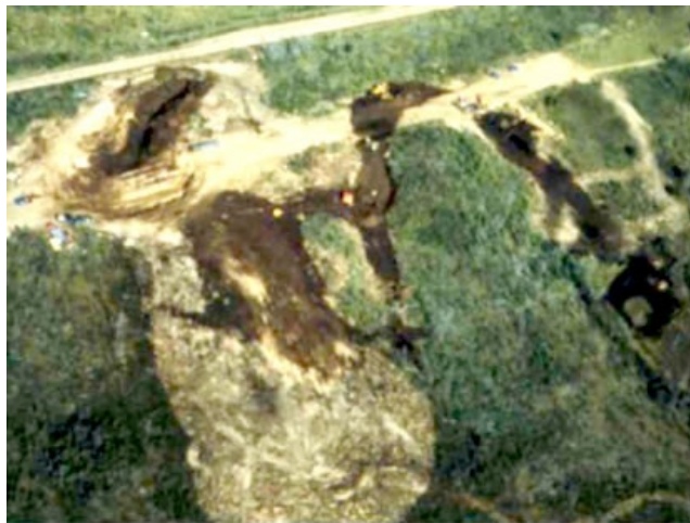
Aerial view of surface oil contamination from the pipeline rupture at the Bemidji Crude Oil Spill Research Site, Minnesota (circa 1979). Much of the black area was caused by oil spraying from the rupture.
