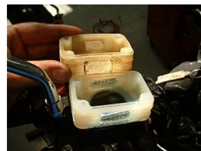
A plastic item with thirty years of exposure to heat and cold, brake fluid, and sunlight. Notice the discoloration, swelling, and crazing of the material
