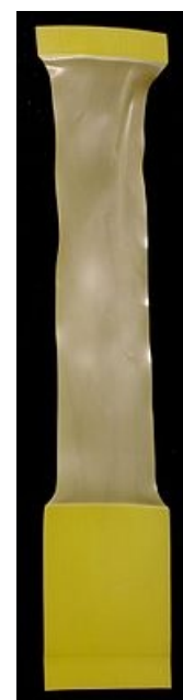
A polyethylene sample that has necked under tension.
