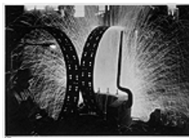
Welding tire rims, International Harvester, Chicago, IL, 1933
