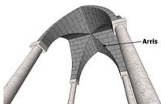
A groin vault (with pointed Gothic profile) viewed from the underside, showing the arris or 'groin'.
