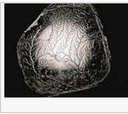
A fractal is formed when pulling apart two glue-covered acrylic sheets
