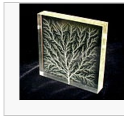
High voltage breakdown within a 4 in (100 mm) block of acrylic creates a fractal Lichtenberg figure
