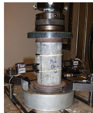
Compression testing of a concrete cylinder
