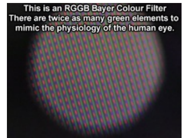
x80 microscope view of an RGB Bayer filter on a 240 line Sony CCD PAL Camcorder CCD sensor
