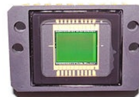
Sony 2/3" CCD ICX024AK 10A 494496 (816*606) pixels CCD removed from Sony CCD-V88E video camera from 1988, with Yellow, Green and Cyan vertical stripe filter
