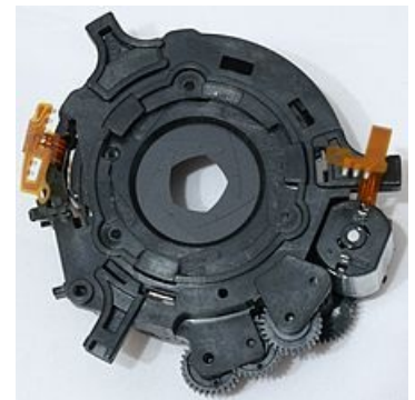
Aperture mechanism of Canon 50mm f/1.8 II lens, with five blades
