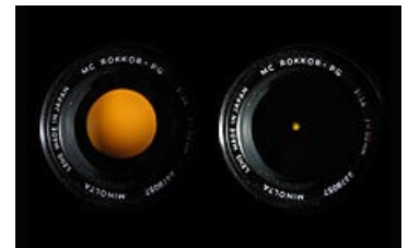
The aperture range of a 50mm Minolta lens, f/1.4 - f/16
