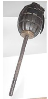
British Mills bomb N°23 Mk II, with rod for launch by rifle
