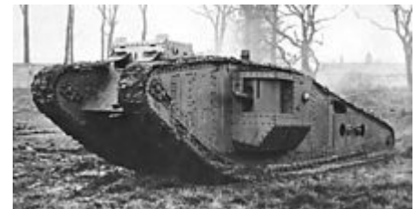
This British Mark IV tank displays a "tadpole tail" extension for crossing especially wide trenches.
