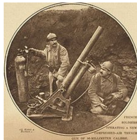
French soldiers operating a compressed-air trench mortar of 86-millimetre calibre
