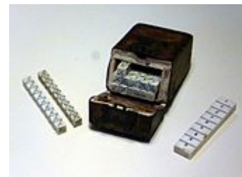
An ivory set of Napier's Bones, an early calculating device invented by John Napier
