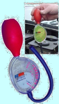
Battery hydrometer - How it works
