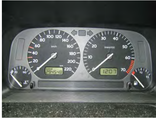
Figure 21.26 The fuel and temperature gauges (far right and far left, respectively) in this 1996 Volkswagen are voltmeters that register the voltage output of “sender” units, which are hopefully proportional to the amount of gasoline in the tank and the engine temperature. (credit: Christian Giersing)
