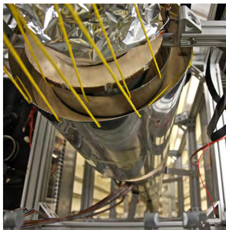
Figure 1.18 An atomic clock such as this one uses the vibrations of cesium atoms to keep time to a precision of better than a microsecond per year. The fundamental unit of time, the second, is based on such clocks. This image is looking down from the top of an atomic fountain nearly 30 feet tall! (credit: Steve Jurvetson/Flickr)
