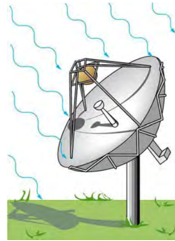
Figure 24.28 Satellite dishes receive TV signals sent from orbit. Although the signals are quite weak, the receiver can detect them by being tuned to resonate at their frequency.
