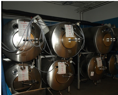
Figure 3. Fermentation of grape juice to make wine produces CO 2 as a byproduct. Fermentation tanks have valves so that pressure inside the tanks can be released.
