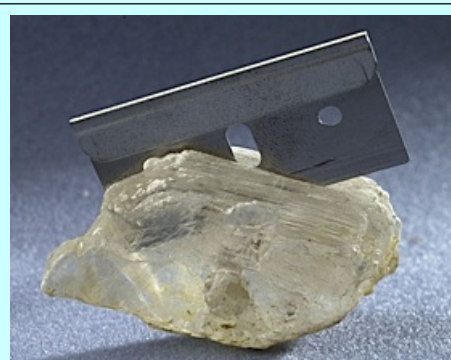
This sample of gypsum ( CaSO_4 ) is easily cleaved with a razor blade. [source]
