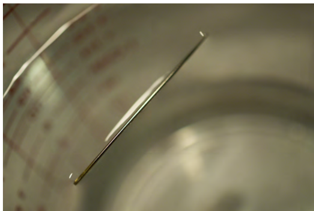
Figure 2.11 The weight of a needle on top of water pulls the surface tension downward; at the same time, the surface tension of the water is pulling it up, suspending the needle on the surface of the water and keeping it from sinking. Notice the indentation in the water around the needle. (credit: Cory Zanker)
