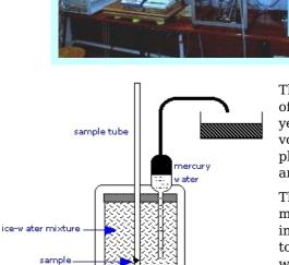
The **ice calorimeter** is an important tool for measuring the heat capacities of liquids and solids, as well as the heats of certain reactions. This simple yet ingenious apparatus is essentially a device for measuring the change in volume due to melting of ice. To measure a heat capacity, a warm sample is placed in the inner compartment, which is surrounded by a mixture of ice and water.
