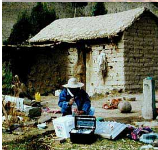
Testing the water quality of SODIS water and raw water with the DelAgua field-test-kit.
