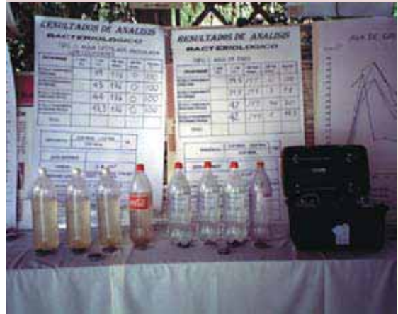
Water quality analysis using a DelAgua field test kit during the workshop to demonstrate SODIS efficiency.
