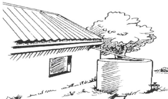
A roof, well maintained gutters and a clean and covered tank are vital in dry regions. (Source: Sustainable Agriculture Manual, IIRR 1998)
